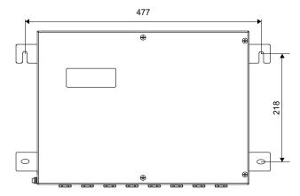
1 - fixing hole for wall mounting Ø 9
