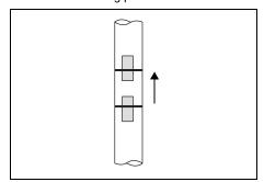
Fig. 3.13: Disadvantageous transducer mounting position
