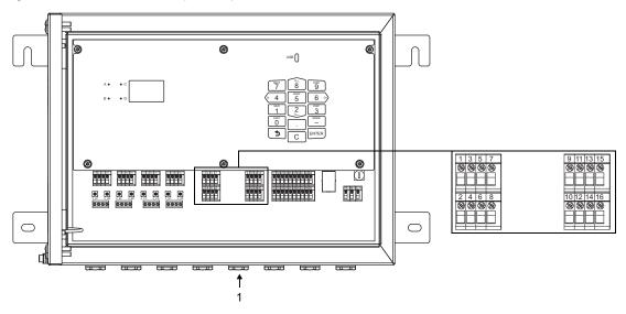
1 - connection of the temperature probe
