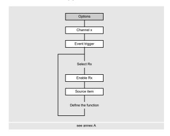
It is possible to configure max. 4 independent event triggers per channel: R1, R2, R3 and R4.
