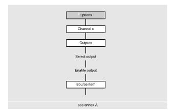
If the transmitter is equipped with outputs, they have to be configured. The measured value, the status value or an event value can be transmitted via the different outputs.
