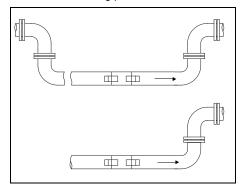
Fig. 3.15: Disadvantageous transducer mounting position
