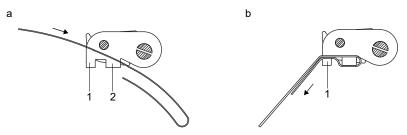
Step 3: Fixation of the tension strap to the pipe
